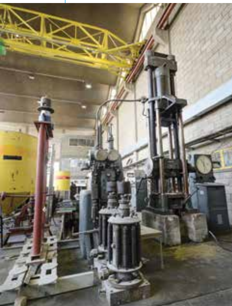
1000kN compression and tension machine and pulsators
